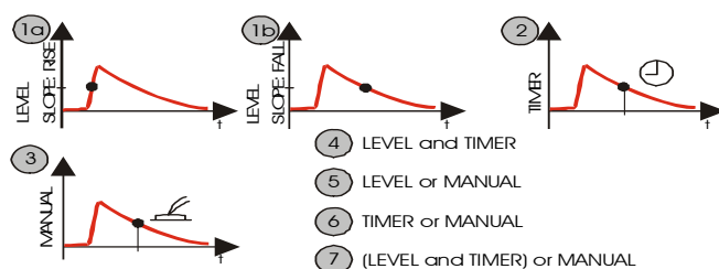
Fig. 54 Triggers for fast logging recording
